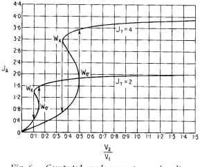
Fig. 6. Computed anode-current—anode-voltage characteristics.
