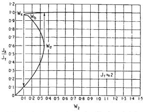
Fig. 7. Anode-current-anode-volts characteristic when k is large.
